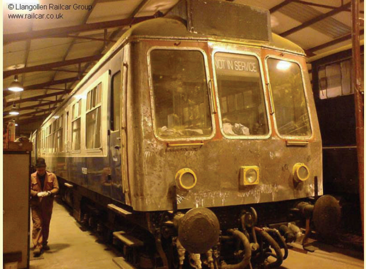
51907 inside the works having cab front repairs. The new sections have been welded in, and the rest of the cab stripped back to bare metal in preparation for a repaint, 20/12/11 (Llangollen Railcar Group)
