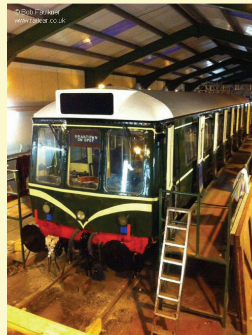
Before, during and after: W51367 is rubbed down and repainted inside the carriage shed at Aviemore during the month of November (B. Faulkner)
