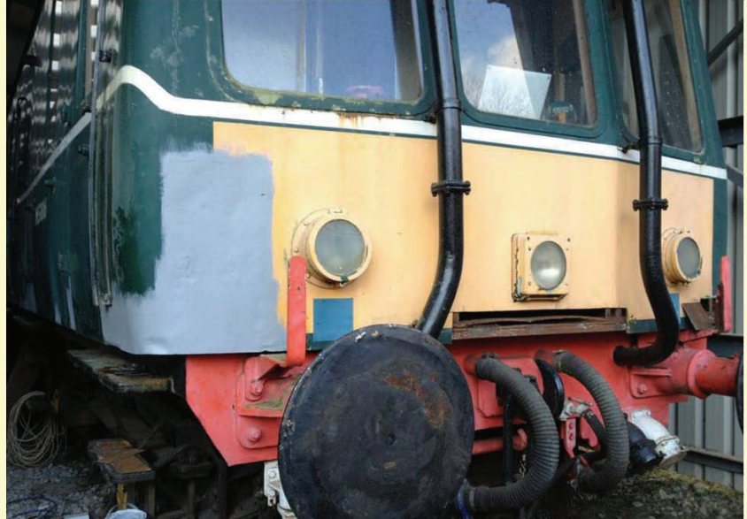
M55006 is receiving bodywork repairs to the cab and lower bodysides over winter (L. Gratton)
